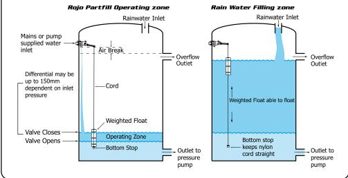
Note: Keep overflow, rain water inlet and outlet to pressure pump as far away from the float valve as possible.
